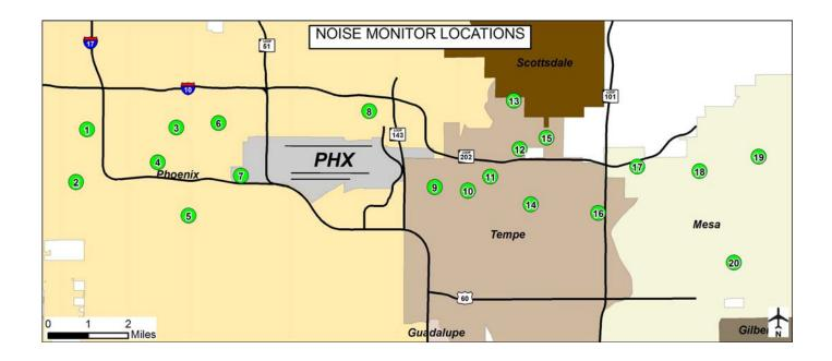
The Aviation Department has 20 Noise Monitoring Terminals (NMT) in the vicinity of PHX. The NMTs are able to determine exactly how loud aircraft operations were at a particular location. In 2009, all monitors were replaced. The new state-of-the-art monitors utilize DSL and Wireless communications which are less susceptible to communication failures than the analog phone lines used in the older monitors.
