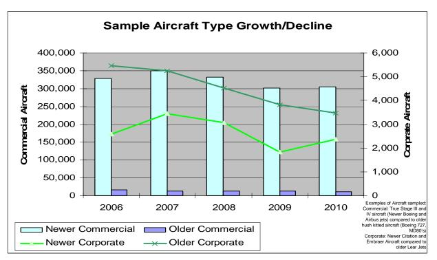
The aircraft fleet mix continues to change as older aircraft are replaced with newer, quieter and more efficient ones. During the past five years, many older aircraft have been retired due to continuing noise concerns, high maintenance and fuel costs. In 2010, newer corporate aircraft made a dramatic increase.
