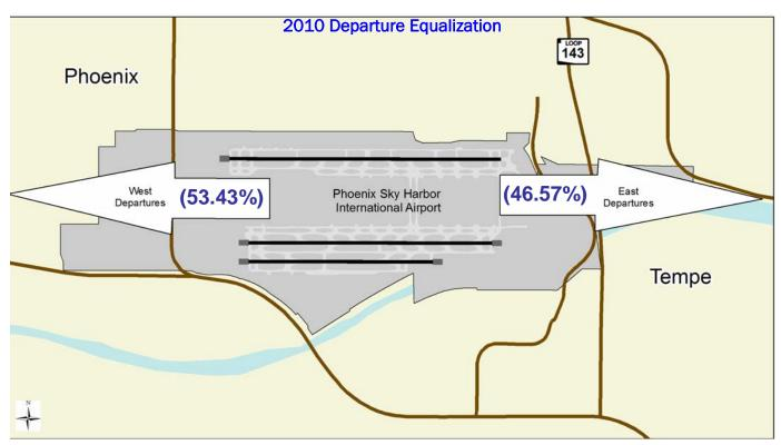
Due to aircraft having to depart into the wind, runway use at PHX is generally predictable with consistent winds. At PHX, winds generally flow east to west at night and, by mid-morning, flow west to east, caused predominantly by solar radiation.
