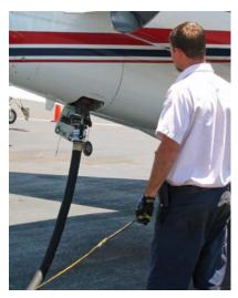
Aircraft fueling vehicles must be equipped with an emergency fuel shut-off that is capable of overriding all other fuel controls and must be able to stop all fuel flow with physical one movement. A deadman control is any device that will stop the flow of fuel when released by the operator. The flow control handle on the nozzle used for overwing fueling is considered a deadman control. Deadman controls must always be used
