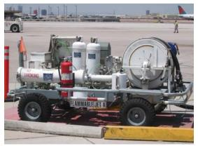
The hydrant fuelservicing vehicle dispenses jet fuel into the aircraft from an underground fuel pipeline network referred to as the hydrant system. The hydrant unit filters the fuel, monitors the gallons pumped, and
