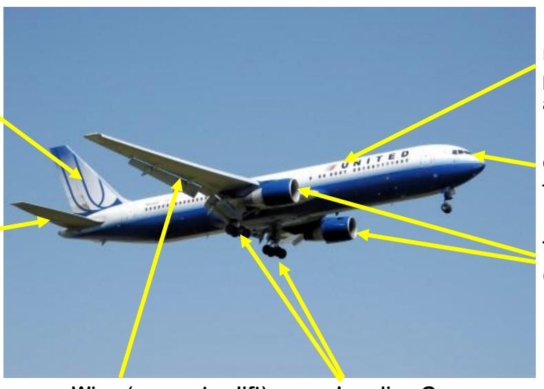
Fuselage (holds passengers, cargo, and fuel)
