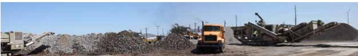
The Airport recycles concrete from runway and taxiway re-construction and uses it as a sub-base for other paving projects. This process is not only sustainable, it saves the Department thousands of dollars per project.
