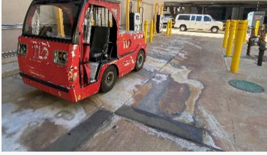
Vehicle Leaking Battery Acid
